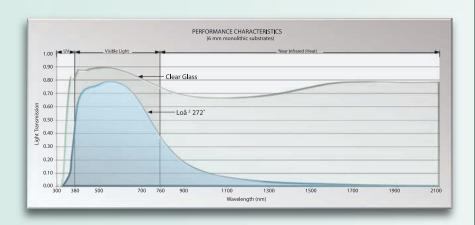
Transmitted and Exterior Appearance of Clearvs. LoE<sup>2</sup>-272 Glass.
