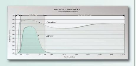
Transmitted and Exterior Appearance of Clearvs. LoE<sup>3</sup>-366Glass
